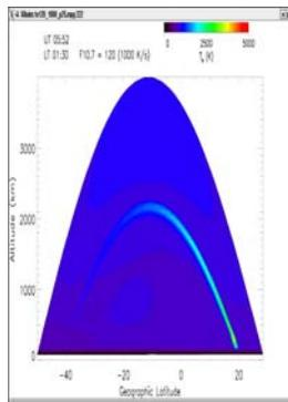
Figure 2: Electron temperature response to ionospheric heating at the Arecibo Observatory, simulation by J Huba (private communication, 2010)
